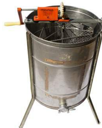
The older tangential 3/6 frame extractor
