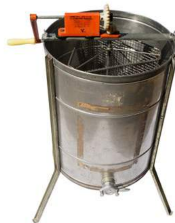
The older tangential 3/6 frame extractor
