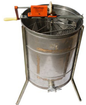
The older tangential 6-frame extractor
