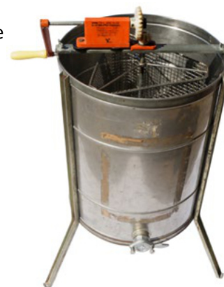
The older tangential 3-frame extractor
